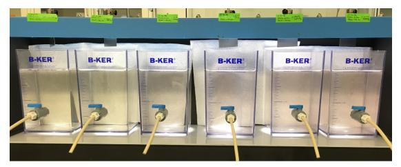
Figure 6-7. Pink water formed after pre-ozonation during Test 3.4. From left to right, jars were pre-ozonated with O3:TOC doses of 0.25, 0.5, 1.0, 1.0, 1.0, 2.0.
