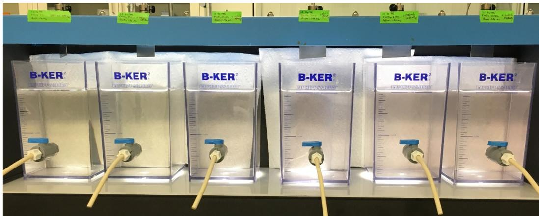
**Figure 6-7. Pink water formed after pre-ozonation during Test 3.4. From left to right, jars were pre-ozonated with O<sub>3</sub>:TOC doses of 0.25, 0.5, 1.0, 1.0, 1.0, 2.0.**
