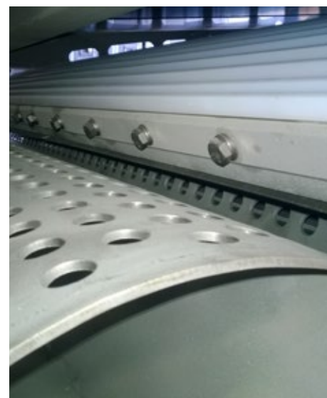
▲ 8 or 12 rolls for lowest residual moisture of final product
